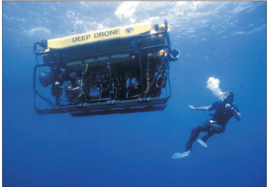
Figure 13-2. Remotely Operated Vehicle (ROV) Deep Drone.
