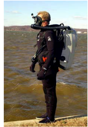
Figure 18-1. MK 16 MOD 1 Closed-Circuit Mixed-Gas UBA.
