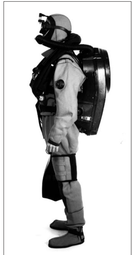
Figure 17-1. MK 16 MOD 0 Closed-Circuit Mixed-Gas UBA.
