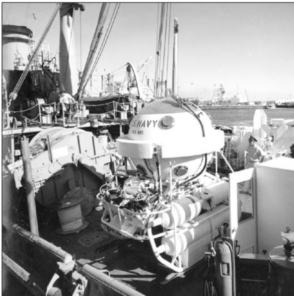
Figure 1-19. DDS MK 1 Personnel Transfer Capsule.
